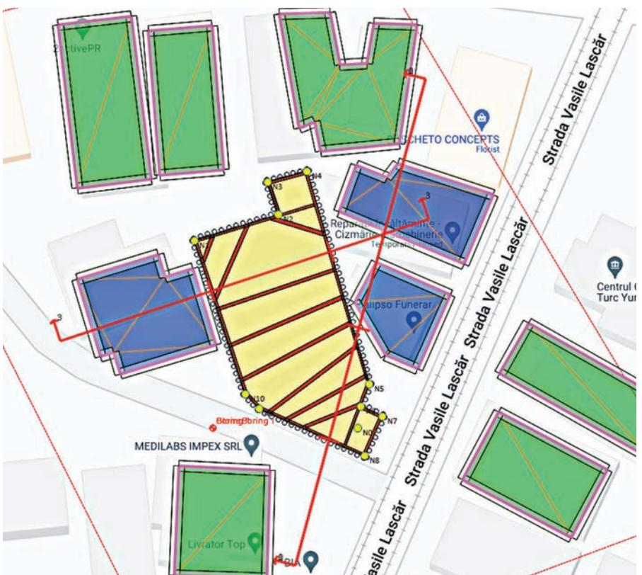
Figure 1: Site map with deep excavation system and twin buildings
