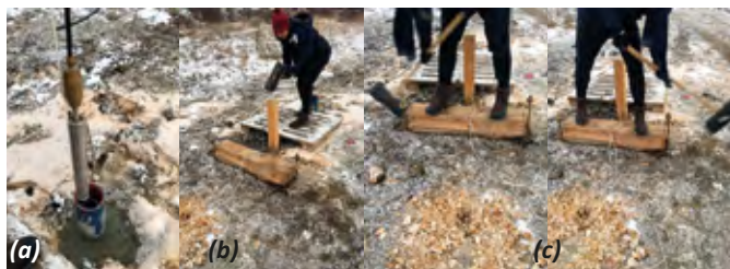
Figure 1: a - borehole sensor for PS logging, b - generation of P-waves, c - generation of S-waves
